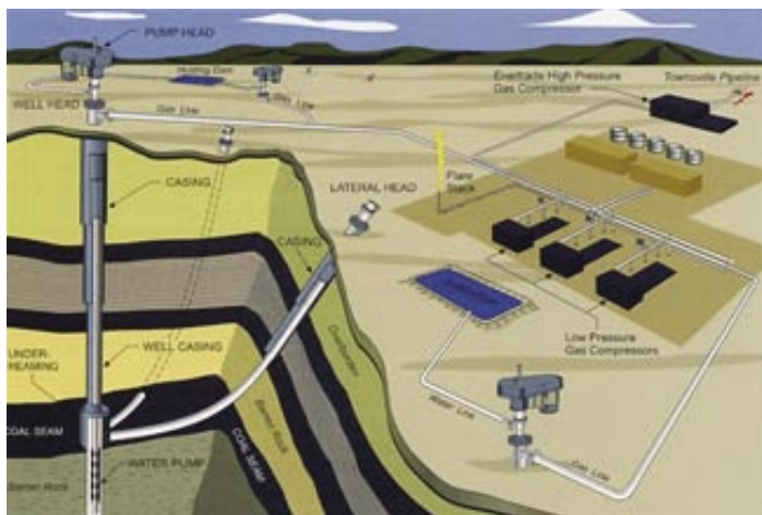
Dymaxion drilling involves both a vertical and horizontal well.
