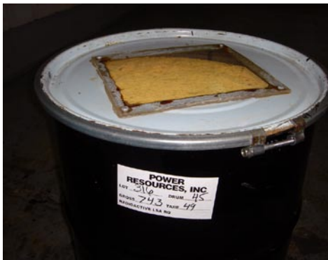
A barrel showing more than 700 pounds of yellowcake, recently produced by Cameco's Power Resources subsidiary at Smith Ranch, near Douglas, Wyoming.
