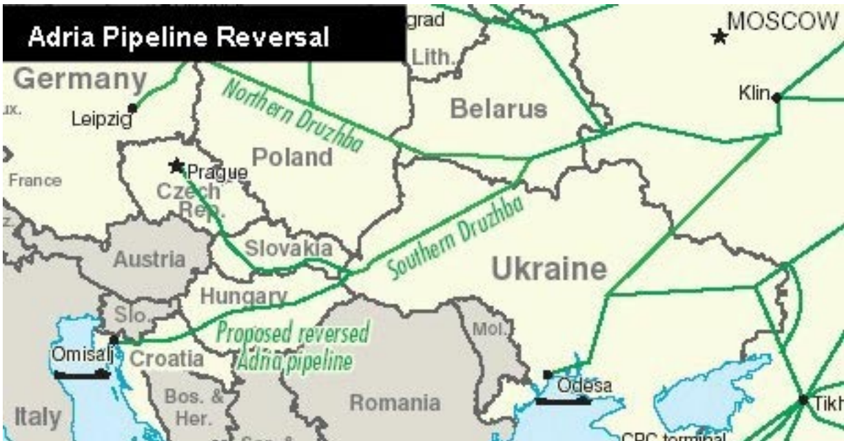
The 2,500-mile Druzhba pipeline, the world's longest pipeline, is the principal daily transport for 1.2 million barrels of Russian and Kazakh oil across Europe. Built in 1964, a recent survey showed 487 damaged points. It needs a major overhaul and more molybdenum. Courtesy of the EIA.
